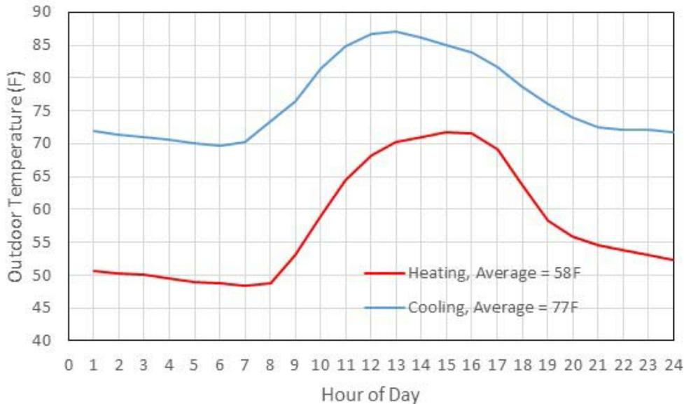
Figure 6. Average day outdoor temperature profile for Cocoa, FL for the days the Outdoor to Indoor flow path experiments were running.
