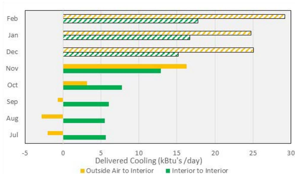
Figure 5. Average daily cooling energy delivered to the building by the HPWH. Hatched bars indicate heating season, solid bars indicate cooling season. Negative values indicate heat was added to the space.
