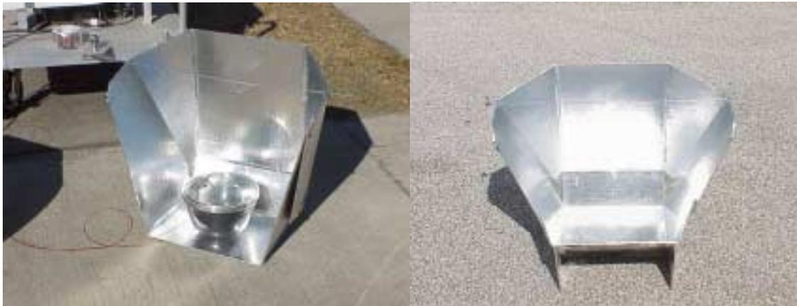
**Figure 6 FSEC/Bernard solar cooker (Note that the cooker on the right has the front reflector)**
