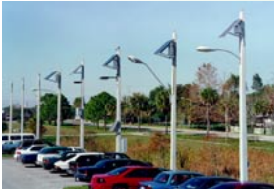
Figure 24. A variety of solar exterior lights undergoing testing at the Florida Solar Energy Center.
