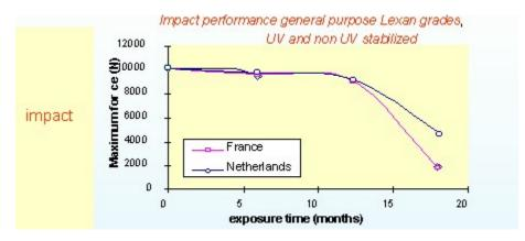
GE also states that *the effect of weatherization is more severe in transparent grades compared with opaque grades*, since many pigments are used in opaque colors that serve to shield the Lexan from UV rays by UV absorption or reflection. Dark colors are more stable than light colors.
