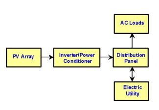
PV systems are and interconnected primary is the systems (PCU). The PCU the PV array into voltage and power grid. and to the grid when directional system AC output network, typically
