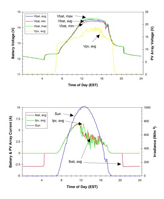
Figure 3-6. Daily operational profile for PV lighting system.
