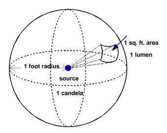
Figure 2-1. Luminous flux and intensity.
