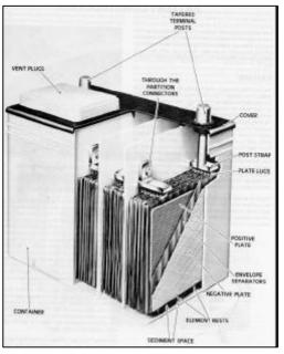
Figure 2-4. Battery cut-away view.
