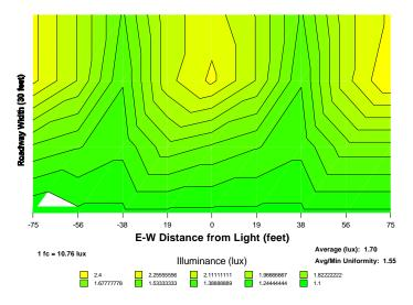
Figure 4-2. Iso-footcandle diagram for roadway lighting application.
