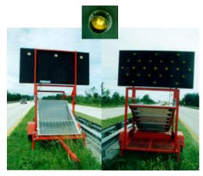
Figure 3-16. PV-powered directional arrowboard.
