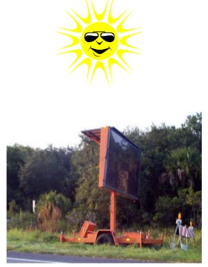
Figure 3-11. PV-powered internally illuminated message board.
