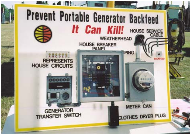
Fig.2: Emergency Power Electrical Connection.
