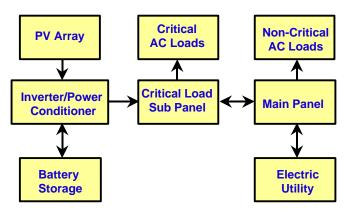
Figure 8. Diagram of grid-connected critical power supply system.
