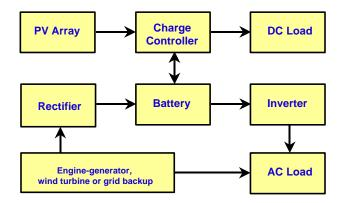
Figure 6. Diagram of photovoltaic hybrid system.
