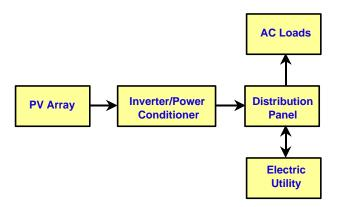
Figure 4. Diagram of grid-connected photovoltaic system.
