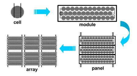
Figure 2. Photovoltaic cells, modules, panels and arrays.
