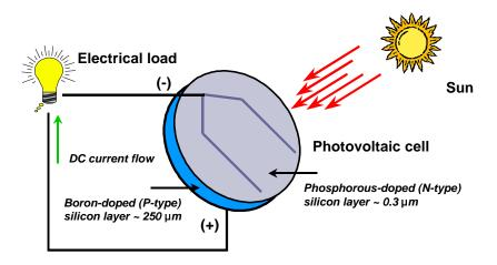
Figure 1. Diagram of photovoltaic cell.
