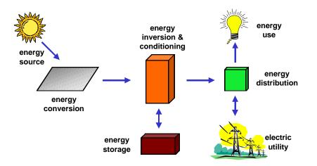
Figure 3. Photovoltaic system components.
