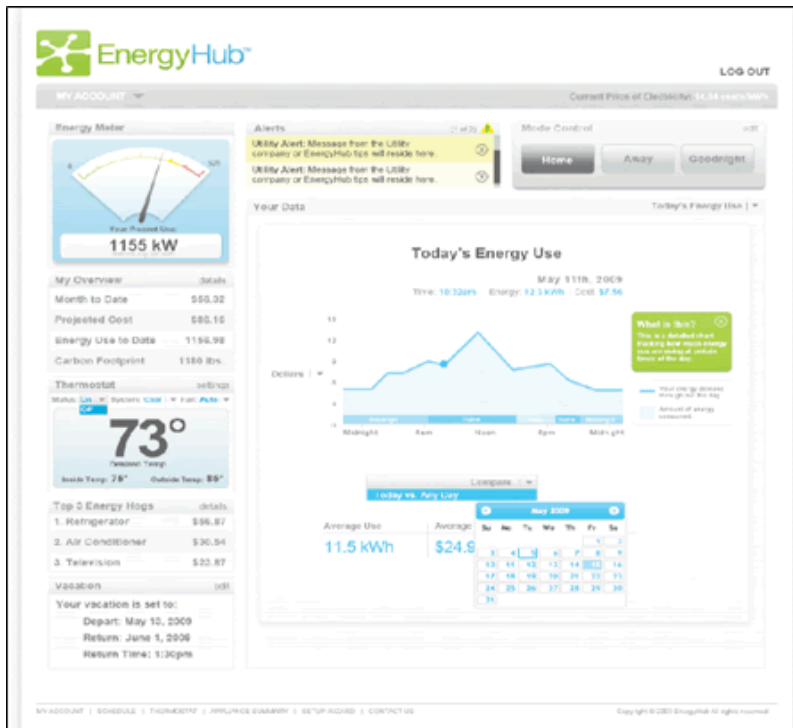
Figure 16. Example of feedback information from the Energy Hub display.
