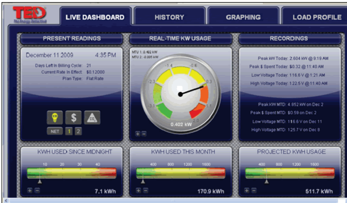
Figure 11. TED 5000 energy use dashboard showing current power use of 0.402 kWh and 7.1 net kWh used since midnight.
