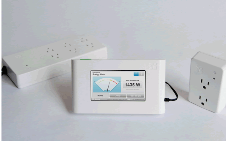
Figure 15. Energy Hub display and outlet control modules.
