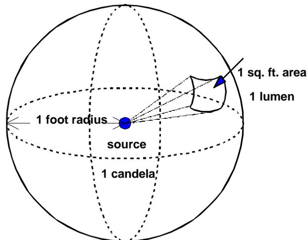
Figure 2-1. Luminous flux and intensity.
