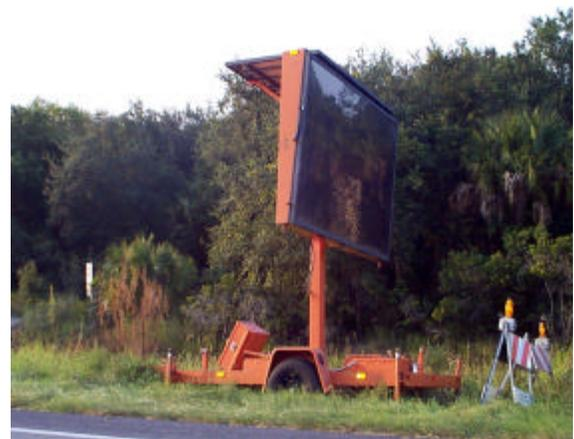
**Figure 3-11. PV-powered internally illuminated message board.**
