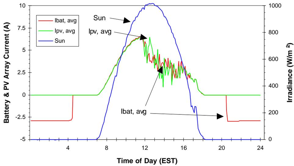
Figure 3-6. Daily operational profile for PV lighting system.
