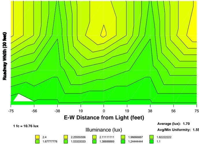
Figure 4-2. Iso-footcandle diagram for roadway lighting application.
