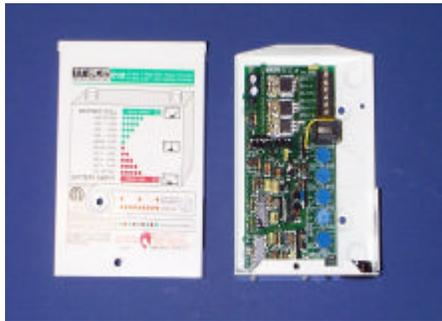
Figure 2-5. PV lighting system controller (Trace Engineering).
