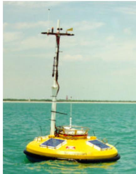
*Figure 3-13. PV-powered ODAS buoy with beacon light.*
