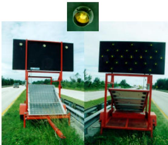
**Figure 3-16. PV-powered directional arrowboard.**
