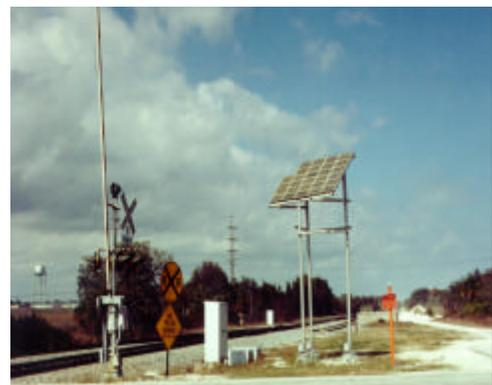
**Figure 3-17. PV-powered railway signals (FEC).**
