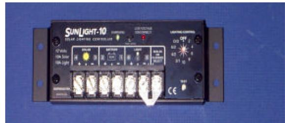
Figure 2-6. PV lighting system controller (Morningstar).
