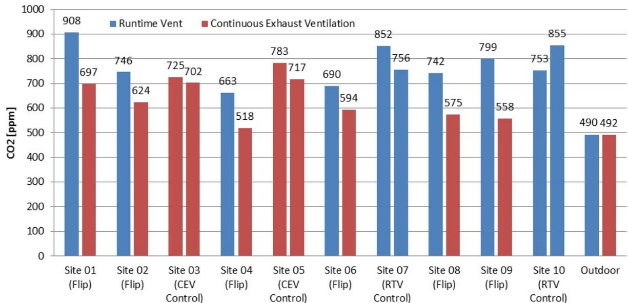
Figure 6. Daily average CO<sub>2</sub> concentration, broken into runtime vent (left bar) and continuous exhaust (right bar) periods. Sites 3 and 5 always operate with continuous exhaust, and sites 7 and 10 always operate with runtime vent.
