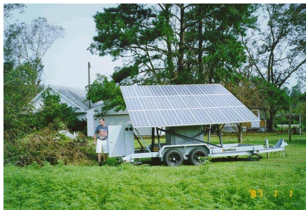
Figure 2. FEMA 1,800 Wp Trailer
