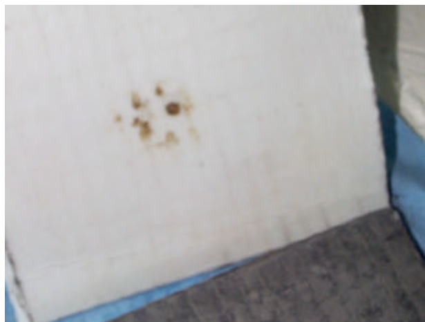
Figure 29. Stain on glass mat between positive and negative cell.
