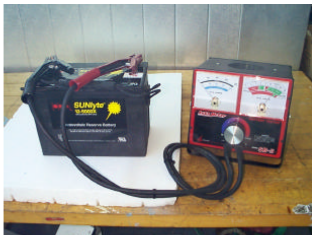
Figure 24. Battery load test.
