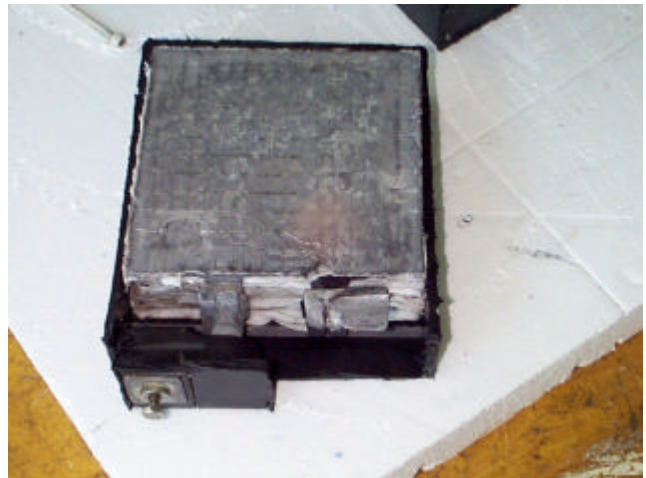
Figure 27. Negative cell extracted from GNB battery 10A.
