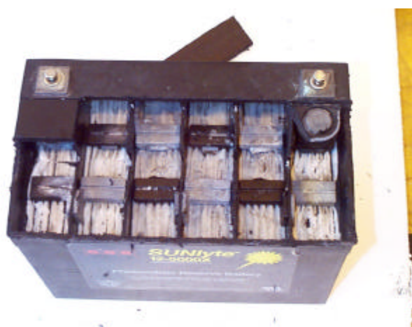
Figure 26. Exposed top of GNB 12-5000X battery.
