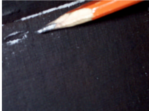
Figure 28. Indentation caused by excess material on positive plate.
