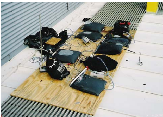
Fig. 3: Test setup of showers
