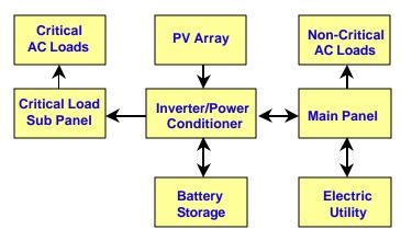
configuration, critical loads are typically supplied from a dedicated load sub panel.
