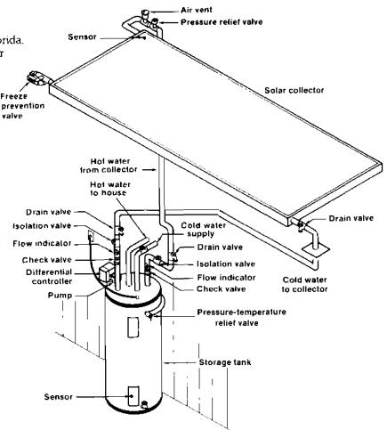
Figure 1. Typical direct pumped system.
