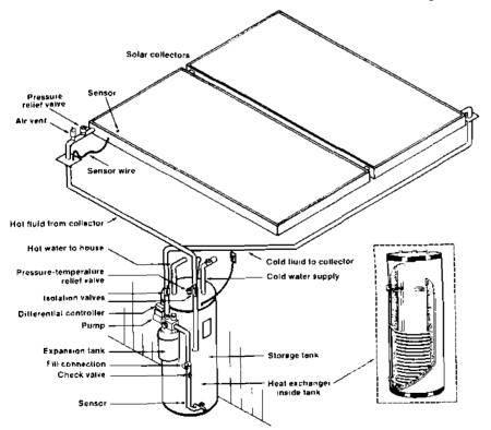
Figure 3. Indirect pumped system using antifreeze solution.
