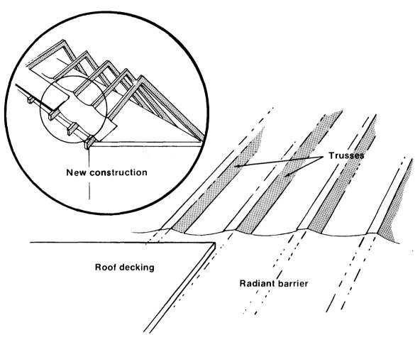
Figure 5. Radiant barrier installation in new construction.
