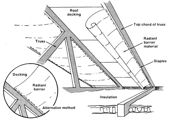
Figure 3. Locations for radiant barrier materials.
