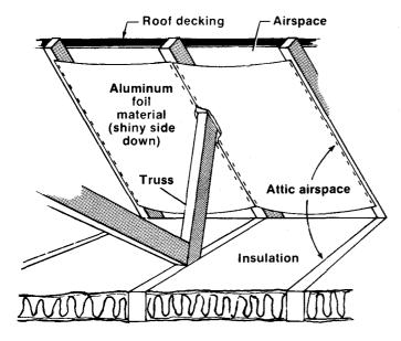
Figure 1. An installed radiant barrier.
