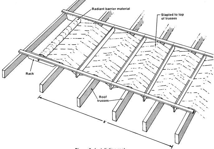
Figure 6. Installation rack.
