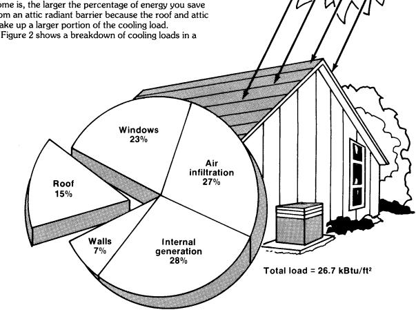
Figure 2. Annual air conditioning load sources for a typical 1500 ft<sup>2</sup> Central Florida home.
