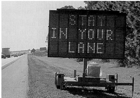
Figure 10. PV-Powered Changeable Message Sign
