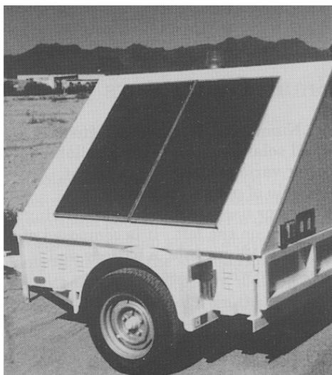
Figure 2. Trailer-Mounted PV Generator
