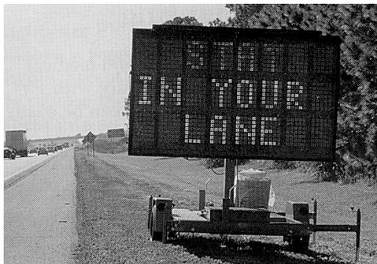
Figure 10. PV-Powered Changeable Message Sign
