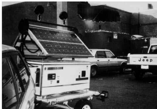
Figure 4. Emergency Mobile Communications and Lighting Unit
