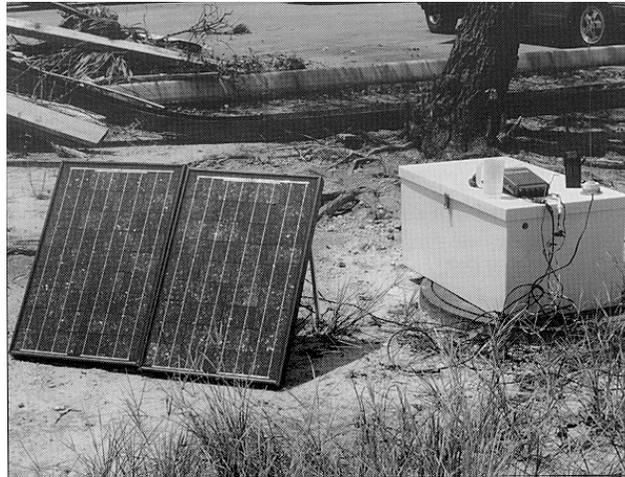
Figure 5. FSEC Training System Powering Amateur Radio Communications
