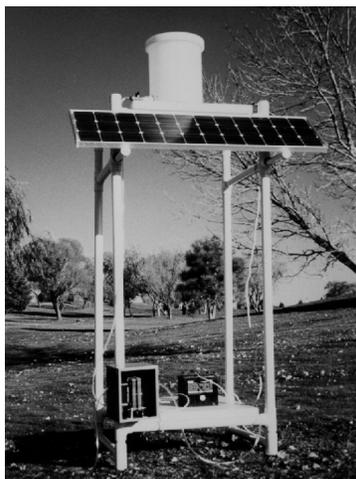
Figure 13. PV Water Purification Unit
