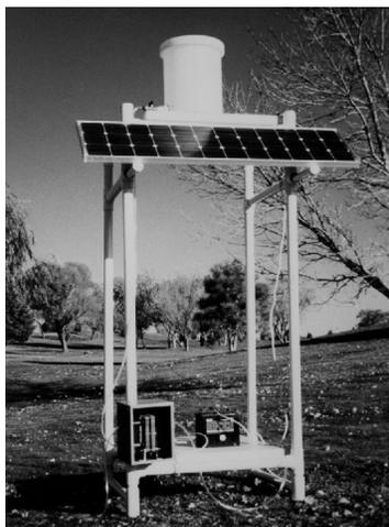
Figure 13. PV Water Purification Unit
