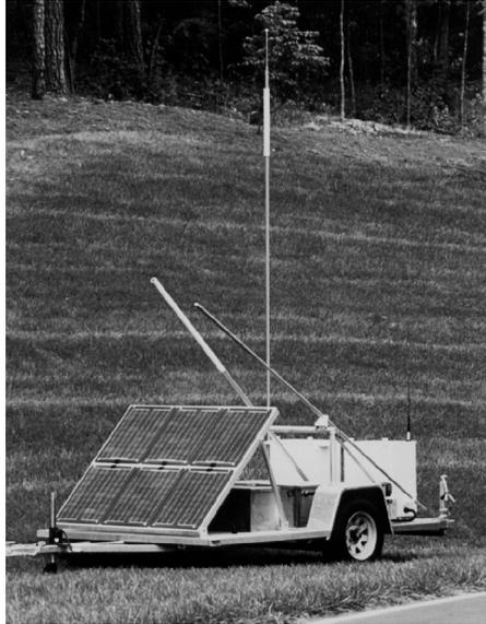
Figure 9. PV-Powered Radio Transmitter Along I-75
