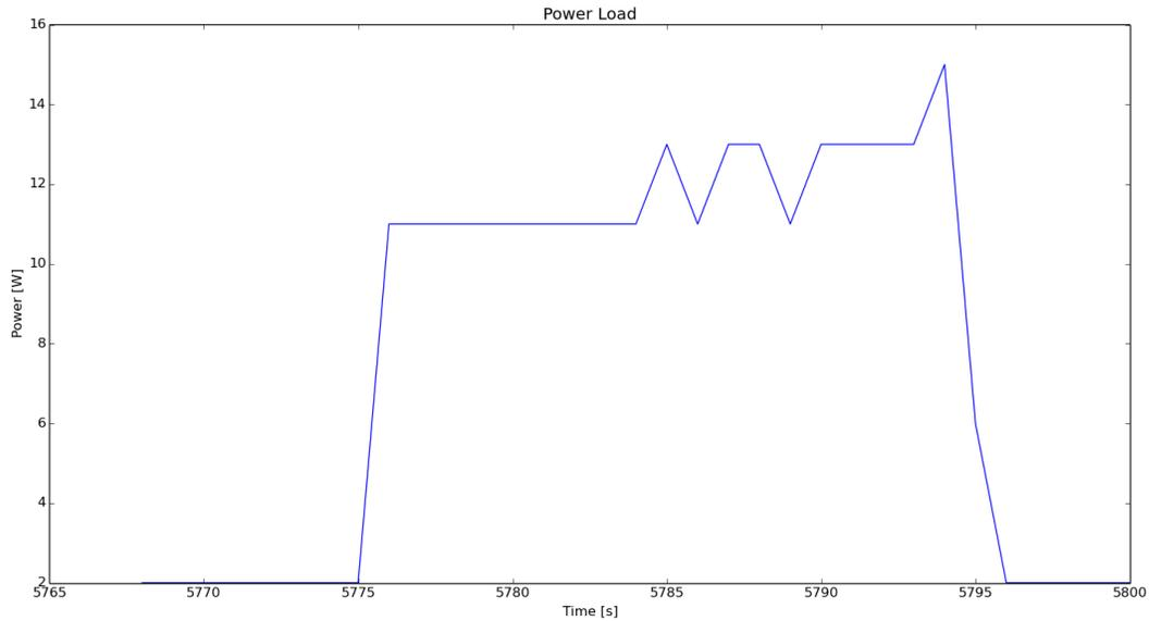
**Figure 5.5:** A particular pattern in the power data is observed when focusing on an individual peak, which can be used as a factor to classify the water boiler in a device database.
