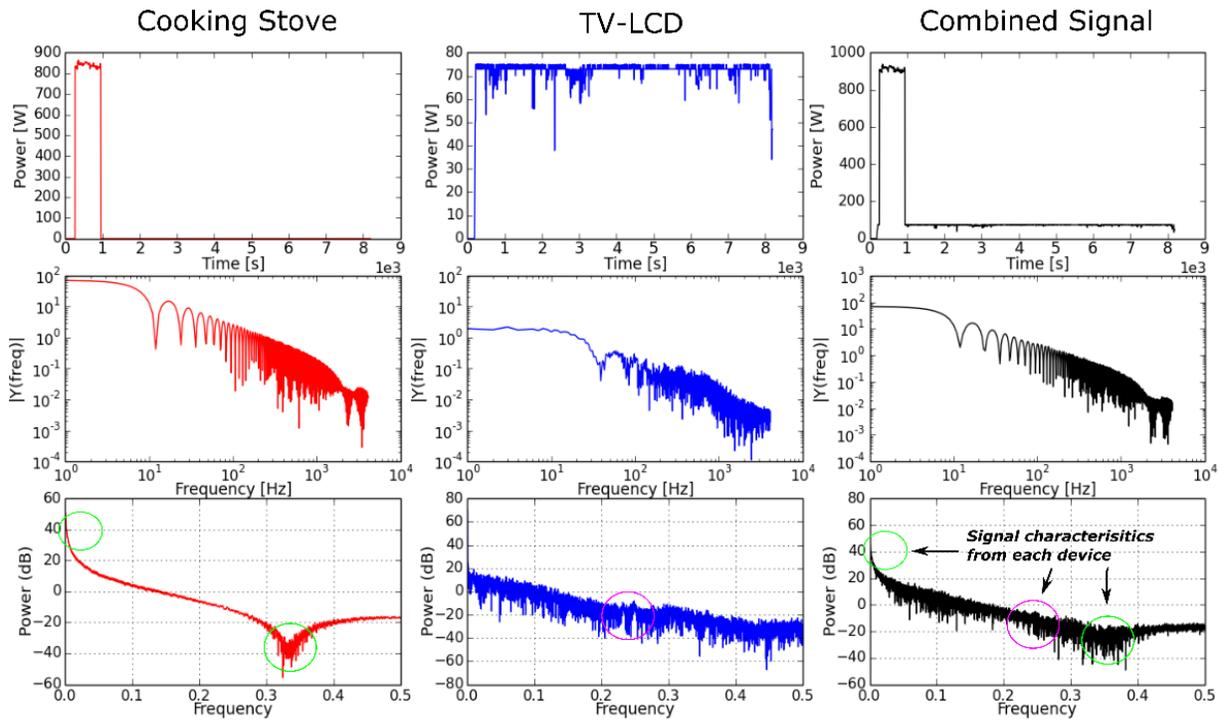
**Figure 5.12:** Column one displays the signal analysis for a cooking stove, column two for a LCD TV, and column three for the sum of the two signals. The green circle shows the location of a specific attribute of the cooking stove PSD signal in the aggregate, while the purple displays the attributes pertaining to the LCD TV.
