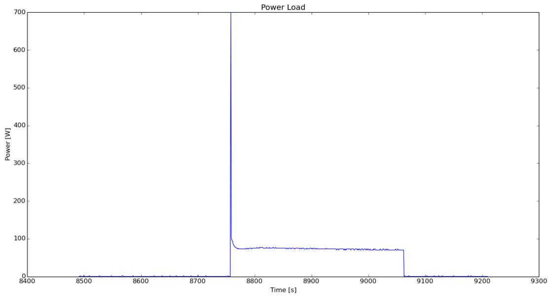
**Figure 5.7:** When focusing on a peak in the plotted power data for the refrigerator, it can be seen that there are defining signal characteristics unique to the device, as was the case with the water boiler in Fig. 12. The unique characteristics were deemed as a factor in recognizing devices in a large collection of power data.
