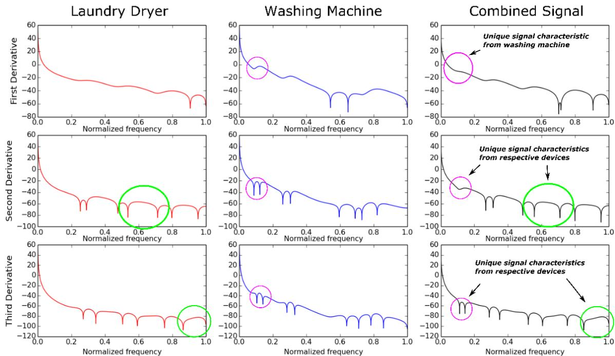
**Figure 5.17:** The first derivative of the washing machine AR PSD shows the influence on the aggregated signal. The second and third derivatives of the device PSDs display even greater influence on the aggregated signals, proving that devices with similar power magnitudes can be distinguished in an aggregated signal.
