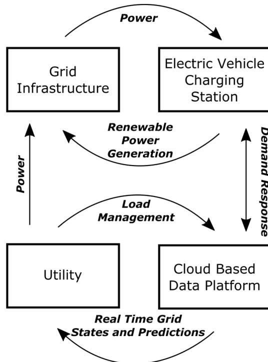
**Figure 3.1:** The system demand structure for a data collection system is presented. A cloud based platform will store and analyze data collected from a home, or business, in real-time, allowing for quick control decisions in demand response programs. One, or several EVCSs, can be analyzed within the urban environment by monitoring the amount of power consumed through the charging station using SPMs.
