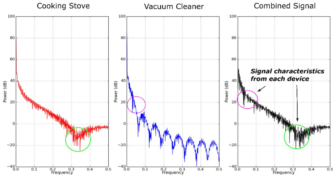
**Figure 5.11:** The implementation of PSD granted the capability to observe unique device signatures that are visible in an aggregated signal.
