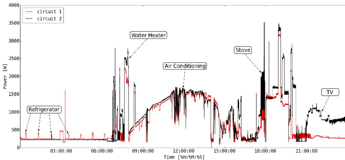
**Figure 5.1:** Devices produce specific power signatures when in use. It can be observed when certain devices are cycled. The cycling of loads within a node displays the behavior and patterns of a consumer that can be used to predict and schedule power generation. Installing a node within a home with an electric vehicle will allow the ability to recognize when an EVCS is in use.
