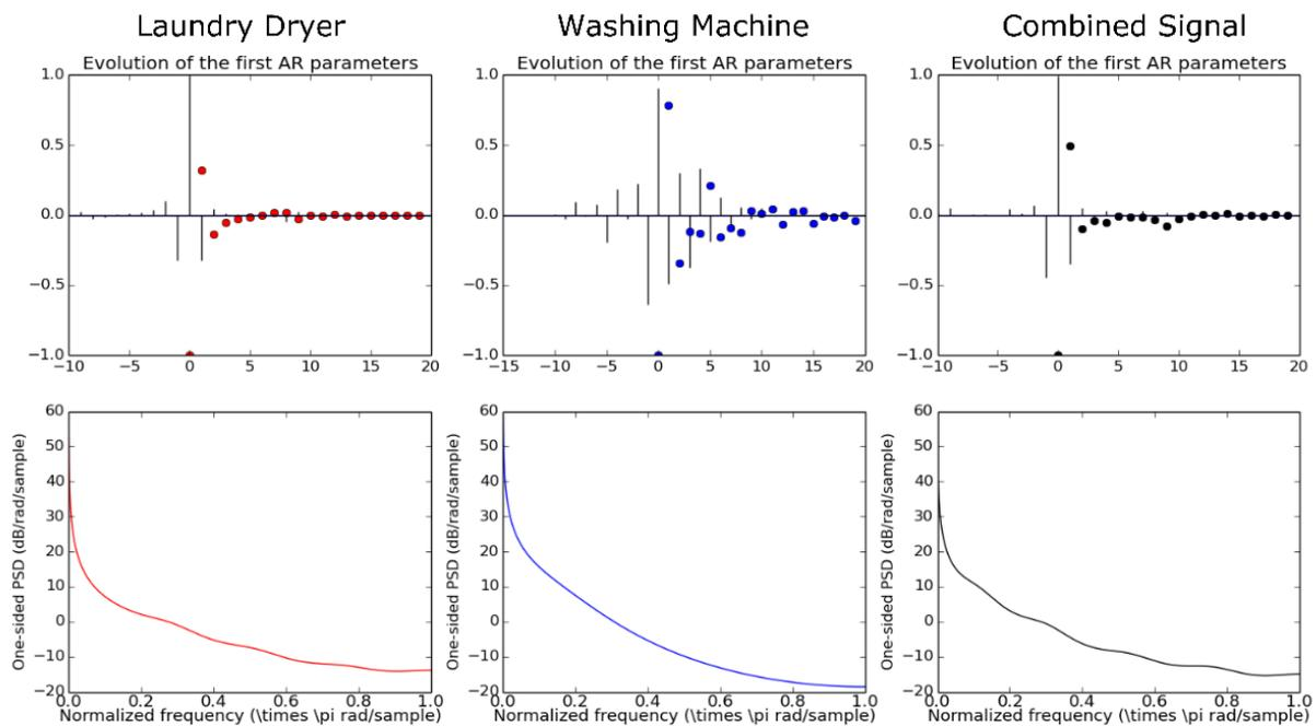
**Figure 5.16:** The AR parameters are plotted in the first row to show to what order they are significant for the respective devices. Defining the order of AR parameters is a necessary step in calculating the correlating PSD plot, which is shown in row two of the figure.
