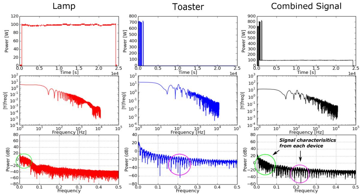
**Figure 5.13:** Column one displays the signal analysis for a lamp, column two for a toaster and column three for the sum of the two signals.
