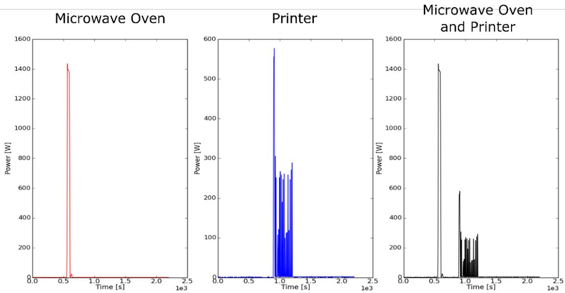
**Figure 5.8:** Two devices can be combined to create a time dependent plot that features both signals, in this case a microwave oven and a printer, however it can be seen that the devices were recorded at different times, so it is necessary to combine the signals into one aggregated signature.
