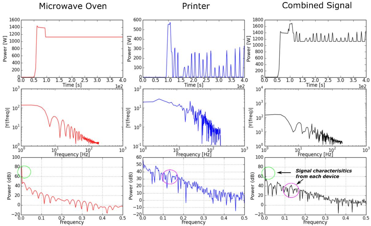
**Figure 5.14:** Column one displays the signal analysis for a microwave oven, column two for a printer, and column three for the sum of the two signals.
