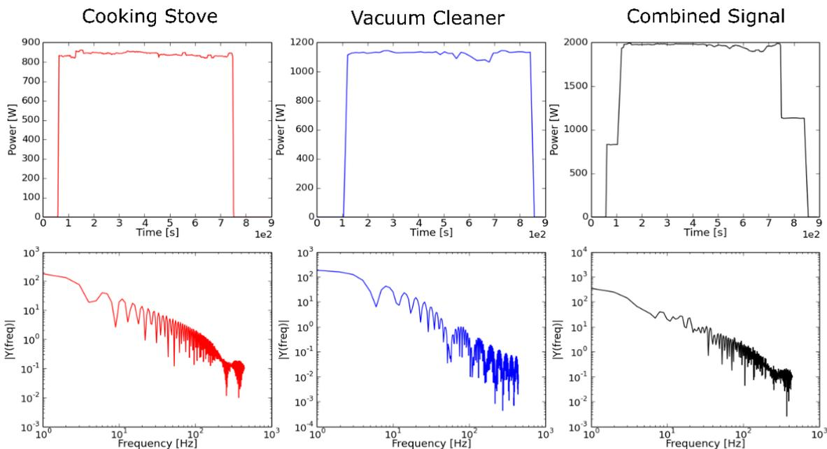
**Figure 5.10:** Once two device signals are combined they can then be analyzed in the frequency domain to better understand if the signals exhibit a specific characteristic pattern.
