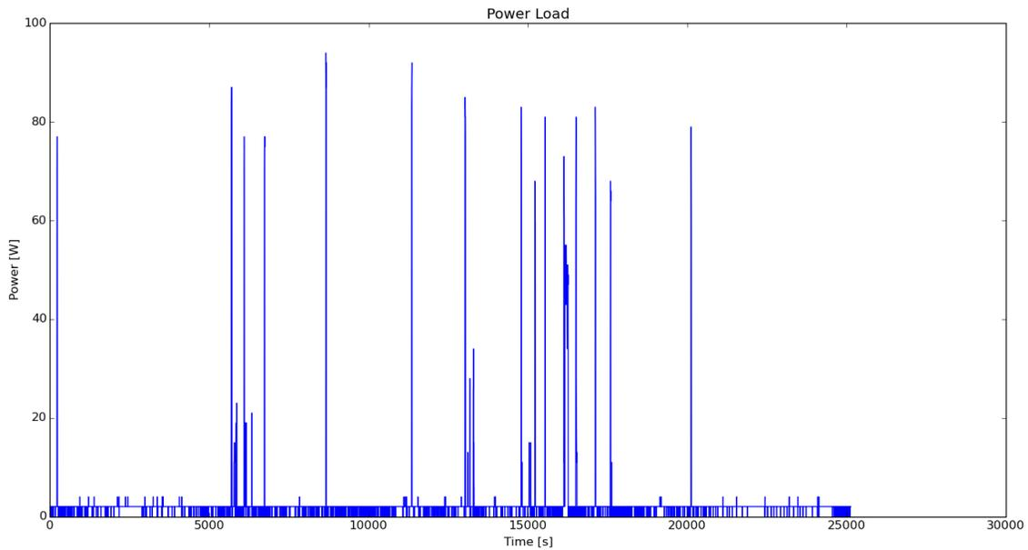
**Figure 5.3:** The cycling of a water boiler is shown. All the measured devices displayed unique power signatures when plotted in the time domain.
