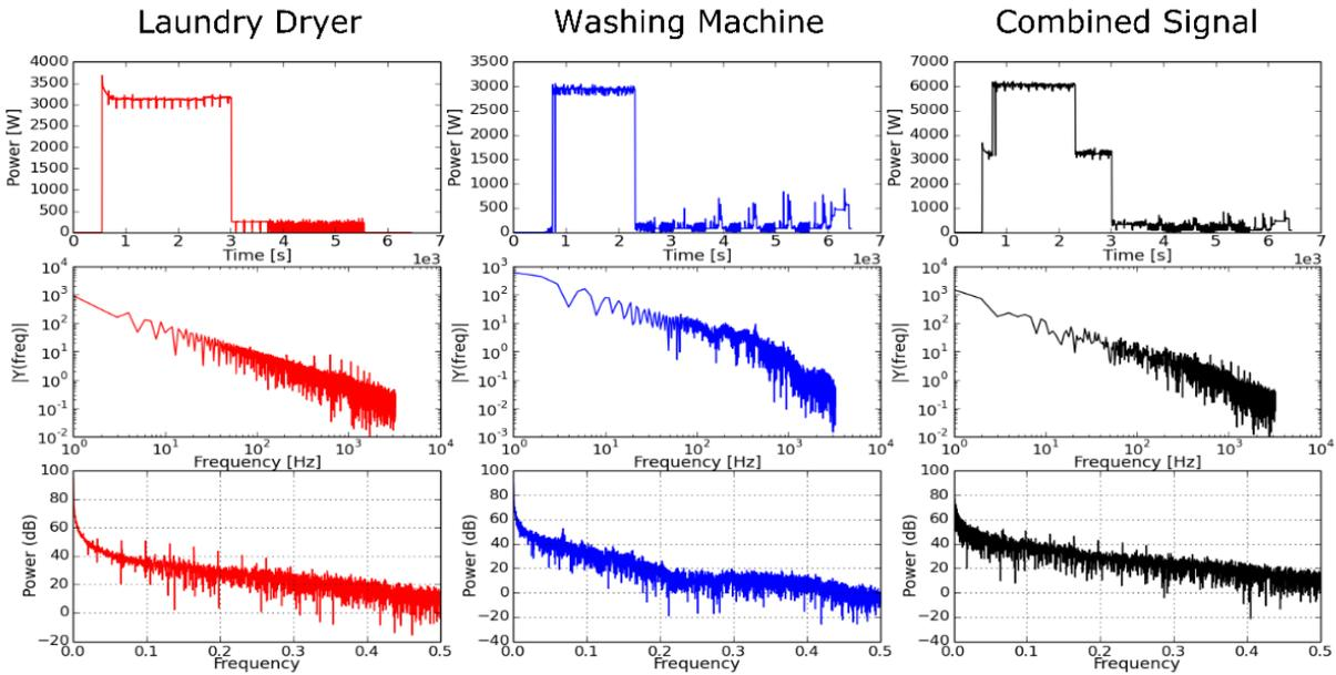
**Figure 5.15:** It can be seen in row three column three that it is not clear which devices make up the signal, so it is necessary to find an alternative method to identify device signatures.
