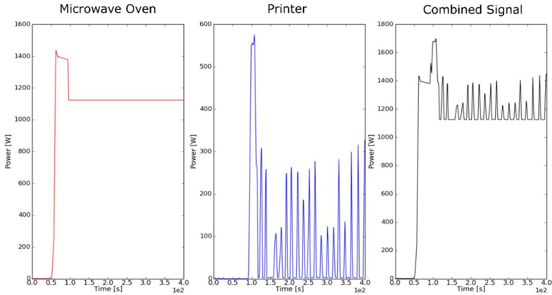
**Figure 5.9:** Aggregating two device signals allows the ability to analyze how the unique characteristics of signals correlating to specific devices interact with each other. Studying this interaction allows the ability to understand techniques for sifting specific devices from a large power set produced by a node.
