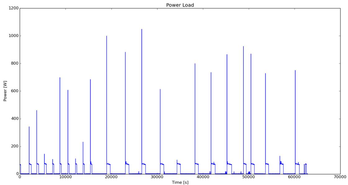
**Figure 5.6:** The power load data for a refrigerator is plotted to display differences between the power signatures of measured devices such as the water boiler in Fig. 5.3.
