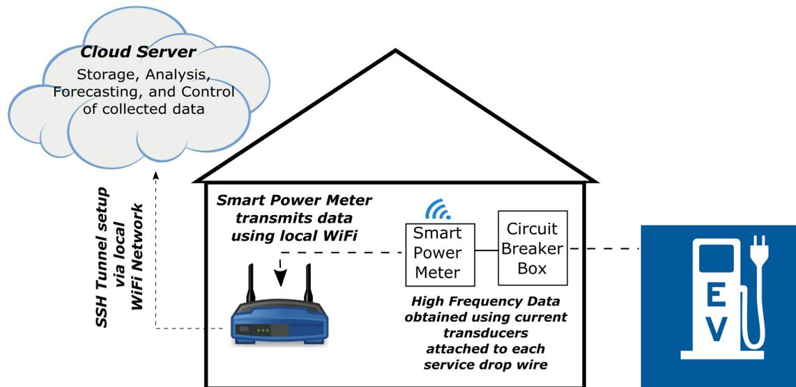
**Figure 3.4:** Utilizing preexisting WiFi connections within a home allow for a cost effective solution for data transmission. Circuit breaker boxes are usually located in a remote area of a building, so it is necessary to utilize a wireless connection to allow for a robust system to monitor and transmit data from a node. A secure SSH connection allows for safe and reliable transmission of data to a server in real-time. The pilot system structure was developed at the University of Hawaii.
