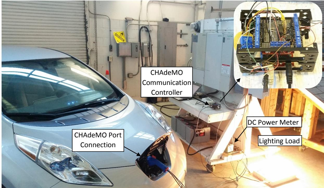
**Figure 8. Operational Micro-grid Application using Electric Vehicle**
