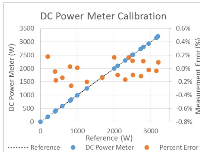
Figure 5. Laboratory Meter Calibration Results
