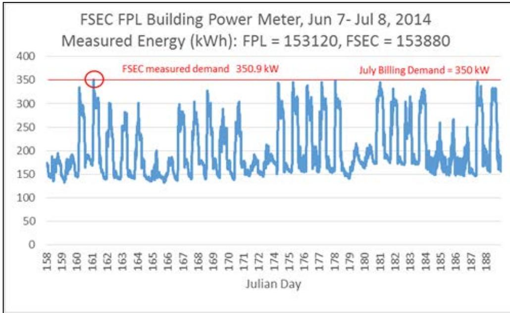
**Figure 3. Comparison of FPL Billing Information to FSEC Measured Energy Use and Facility Demand**
