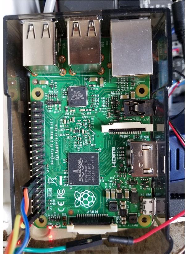
**Figure 2. Raspberry Pi 2 Miniature-Computer for Parallel Measurement and Control**
