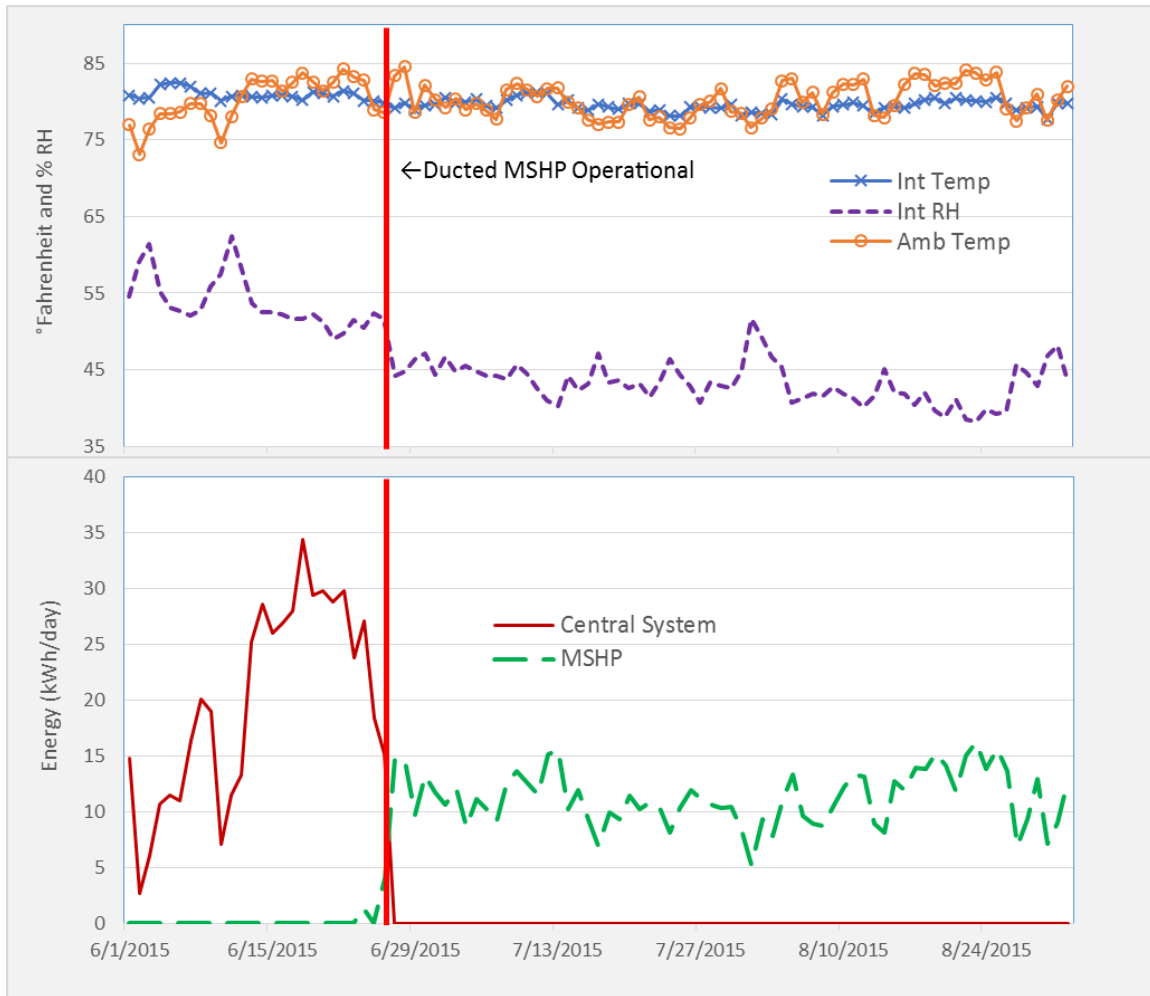
Figure 28. Daily average HVAC energy, indoor and outdoor conditions from June 1, 2015, through August 31, 2015, for Site 61
