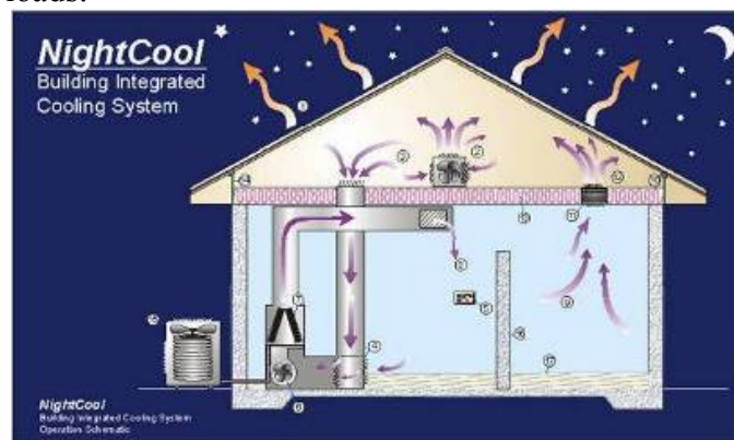
Figure 2-48 NightCool Operation Schematic
