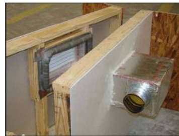
Figure 1-5: Southern Energy Homes Interior Crossover Duct Mockup
