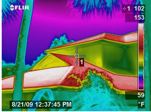
Figure 4-24: Infrared image of the house during midday after mostly sunny conditions all morning.
