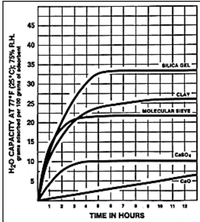
Figure 28. Comparative water adsorption capacity at 77°F against time for various desiccants.
