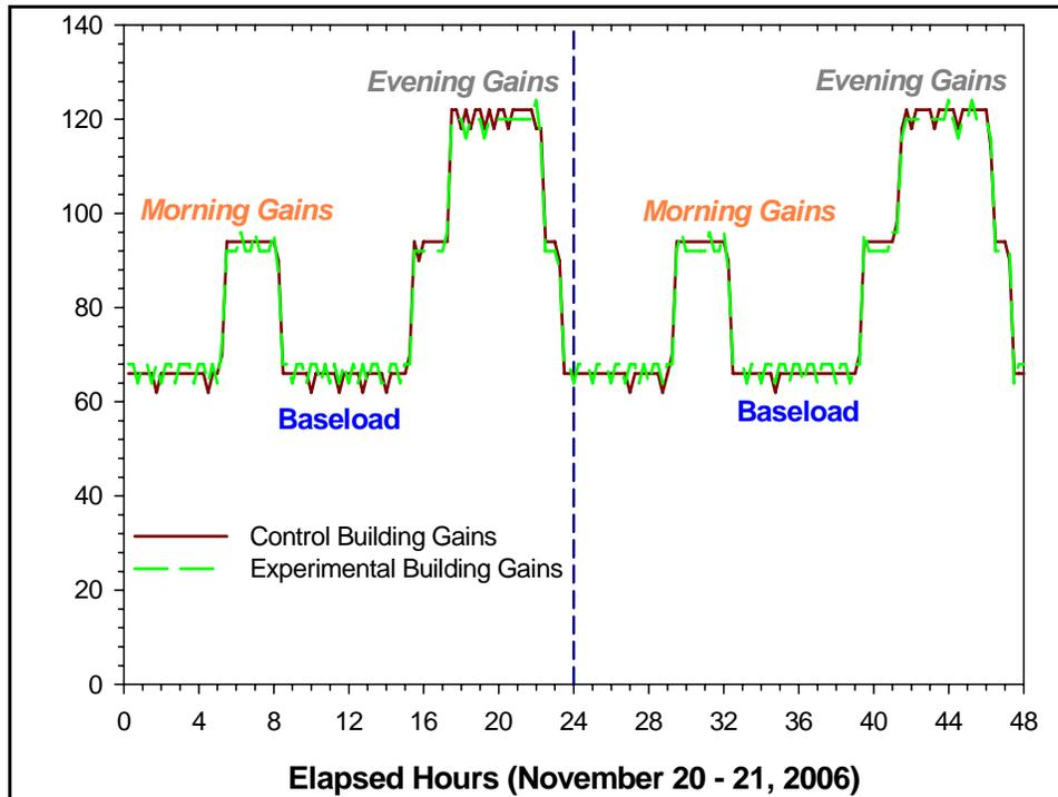
**Figure 11.** 24-hour measured internal gains schedule for *NightCool* test buildings (Watts).
