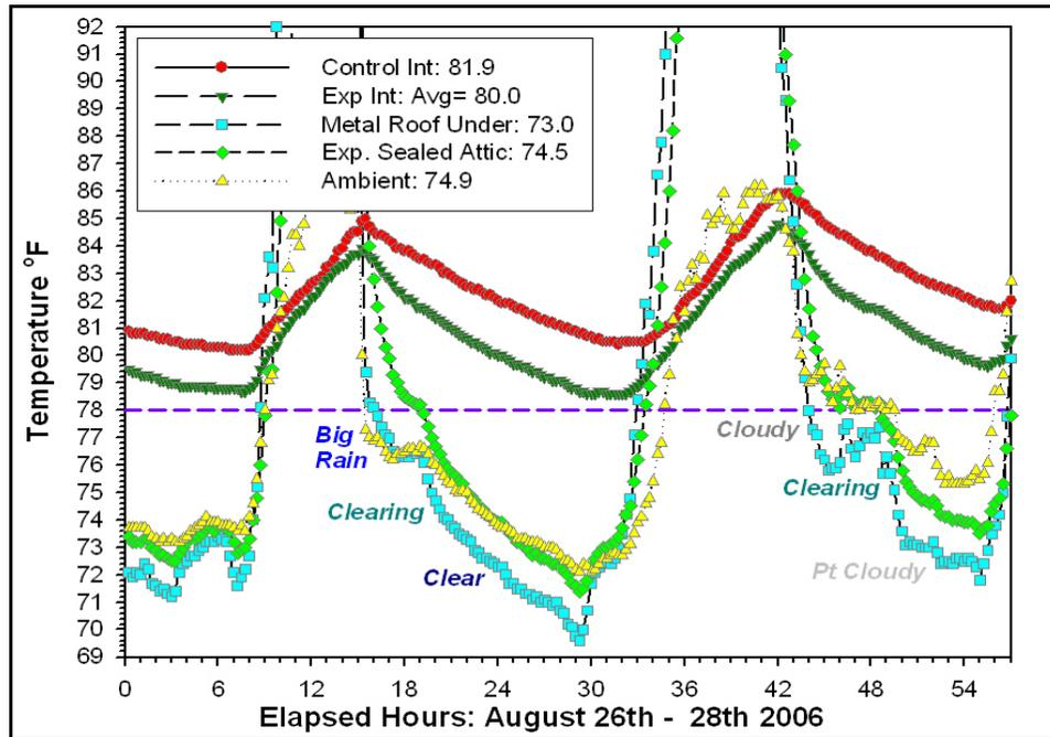
**Figure 13.** *NightCool* by natural convection only: comparative interior temperatures Control and *NightCool* test buildings free float condition (avg. temps from 8PM to 8AM).
