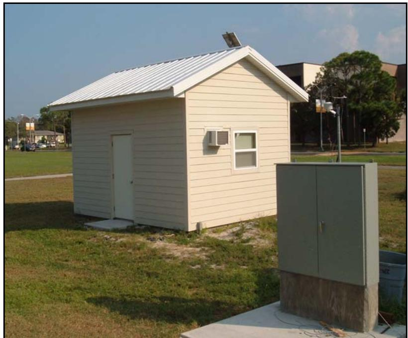
**Figure 15.** Experimental *NightCool* building showing central data acquisition system and wall-mounted air conditioner.
