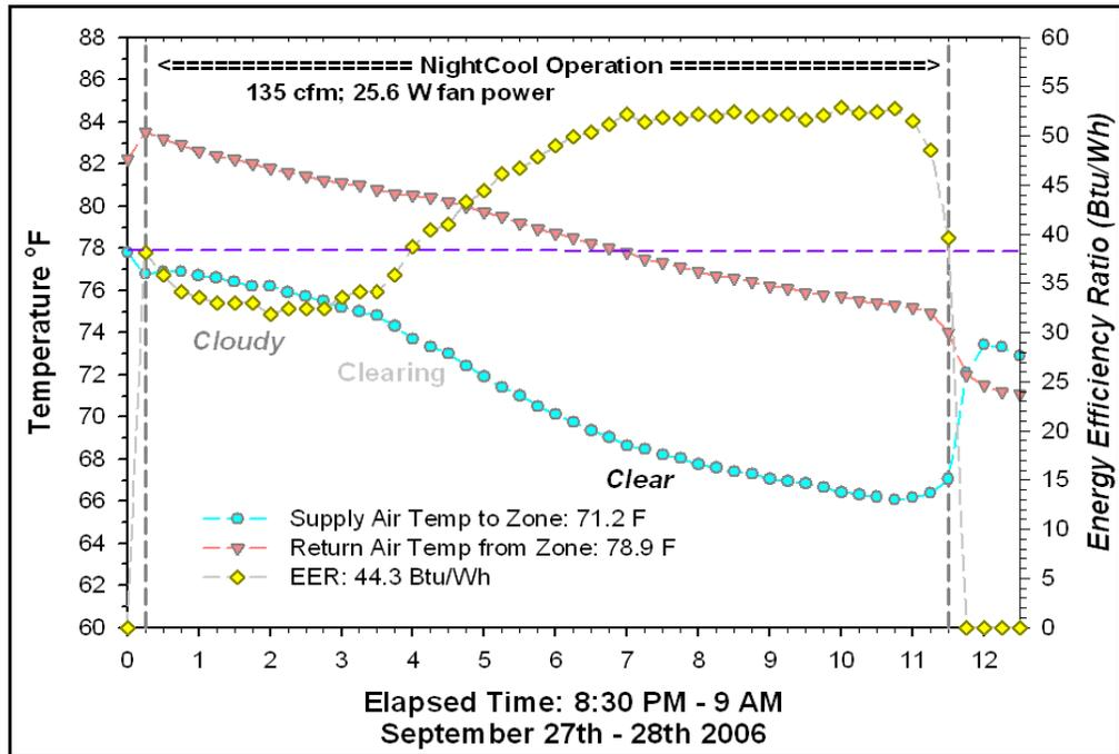
**Figure 17.** *NightCool* system performance with circulation fans operating, but no air conditioning. Supply and return temperatures are shown along with 15-minute system EER.
