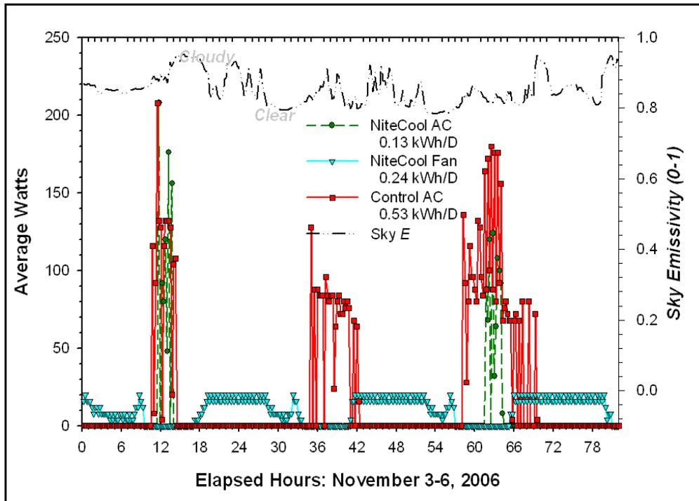
Figure 23. *NightCool* energy performance under mild conditions.
