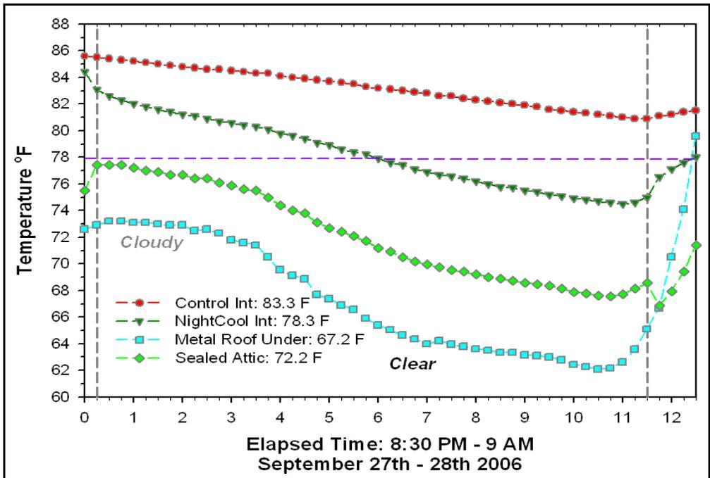
**Figure 16.** *NightCool* thermal performance with fans operating but no air conditioning. For comparison control building interior temperature is shown in red; *NightCool* temperature is green triangles.
