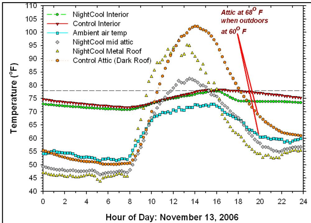
**Figure 32.** *NightCool* performance; clear cool conditions. Note potential for heating during late winter afternoons when outdoor temperature is 60°F.
