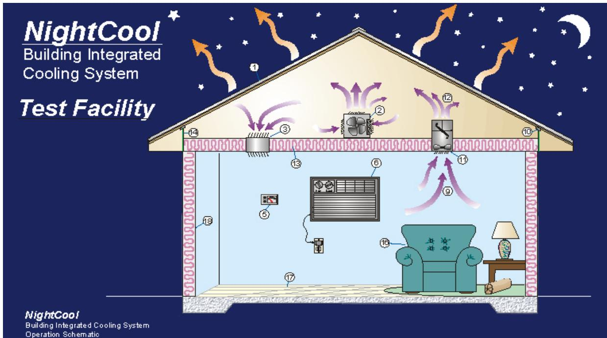
**Figure 2.** *NightCool* test building schematic.
