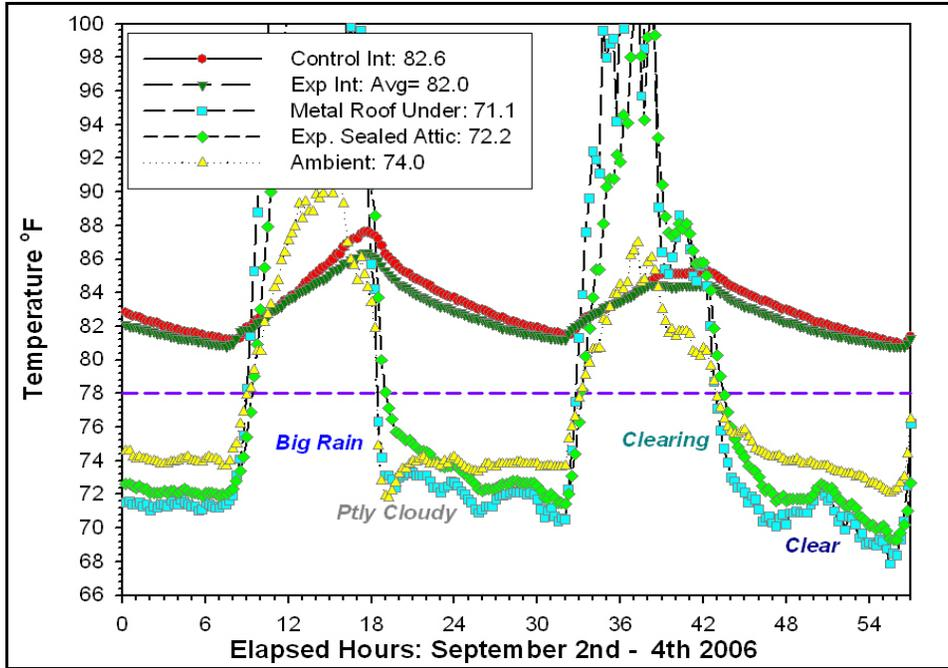
**Figure 12.** Null Test: comparative interior temperatures Control and *NightCool* test buildings; Free Float: no attic convection (avg. temps from 8PM to 8AM).
