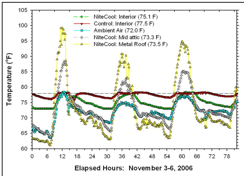
**Figure 22.** *NightCool* thermal performance under mild autumn-like conditions. Note that the *NightCool* building was maintained at a substantially cooler temperature.
