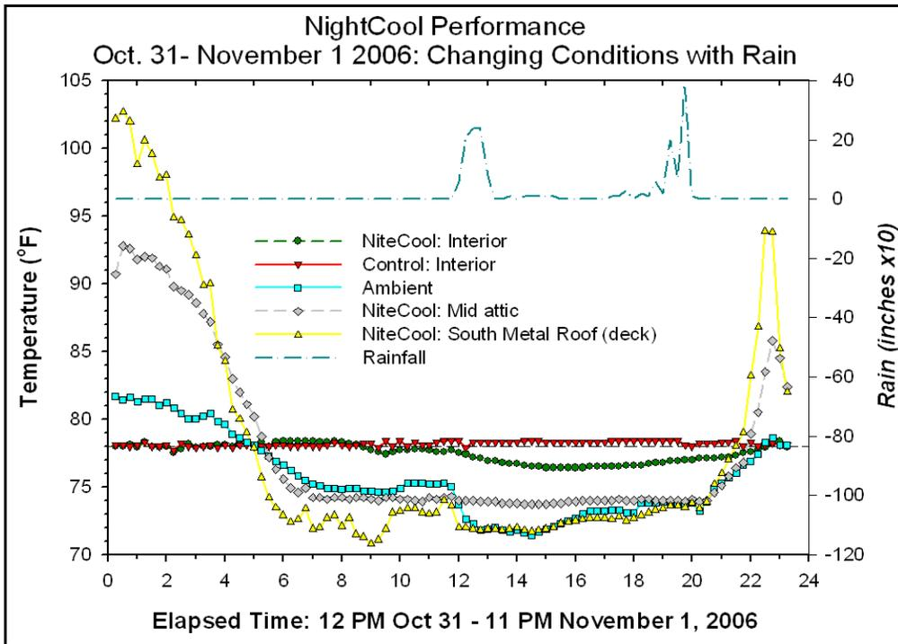
Figure 20. Temperature conditions on interior of *NightCool* and Control building, ambient air temperature and *NightCool* attic/roof.
