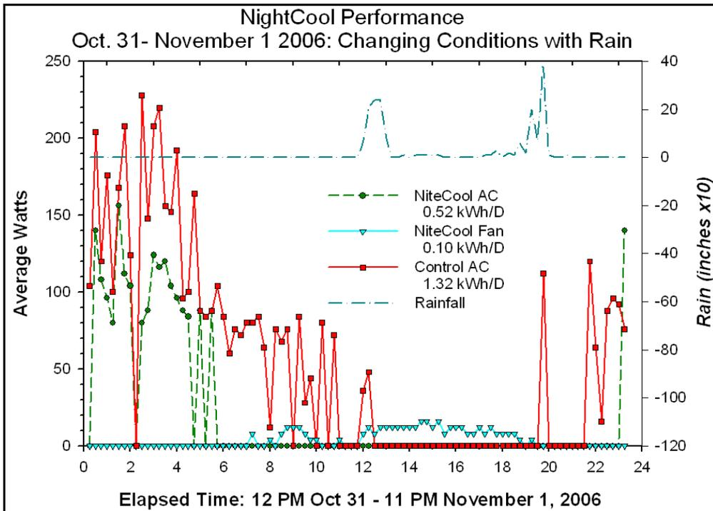
Figure 21. Comparison of AC and *NightCool* fan power with AC power in the control.
