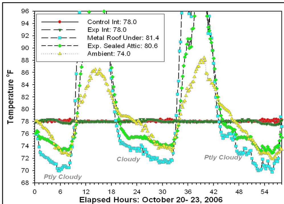
**Figure 18.** Comparative interior temperatures in control and *NightCool* test buildings. AC in both buildings; *NightCool* in experimental.
