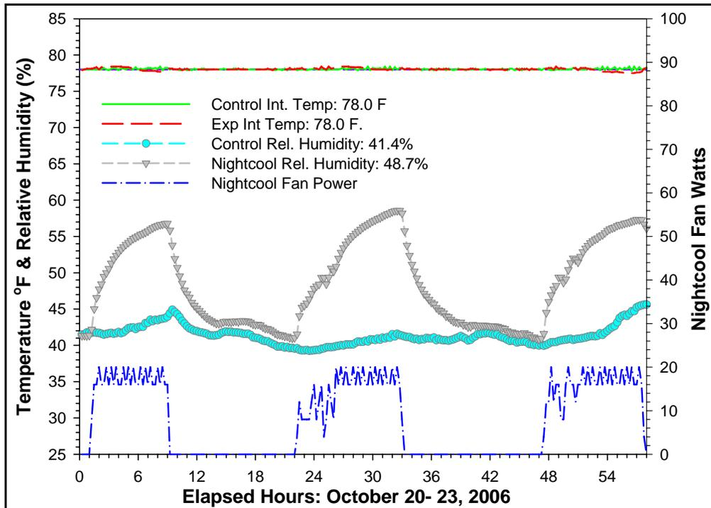
**Figure 26.** Comparative interior relative humidity in control and *NightCool* test buildings. AC is used in both buildings, but *NightCool* is activated at night in the experimental facility.
