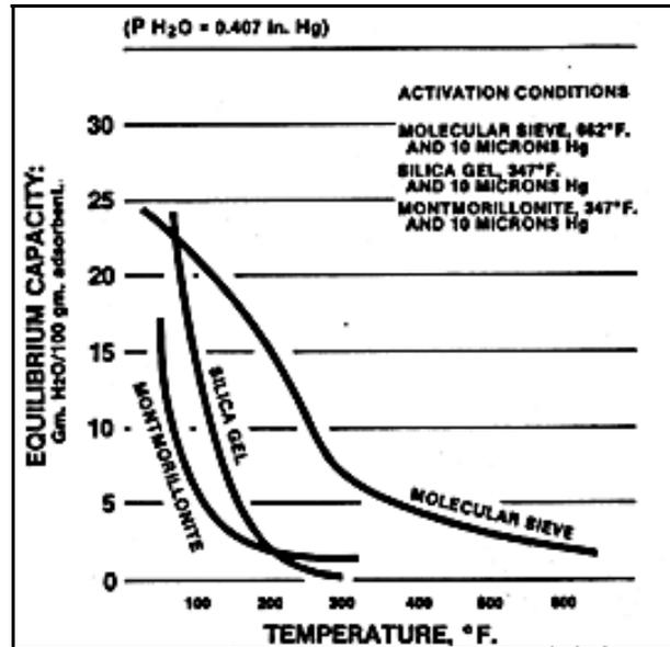
Figure 29. Equilibrium moisture capacity of clay vs. other desiccants against environmental temperature.
