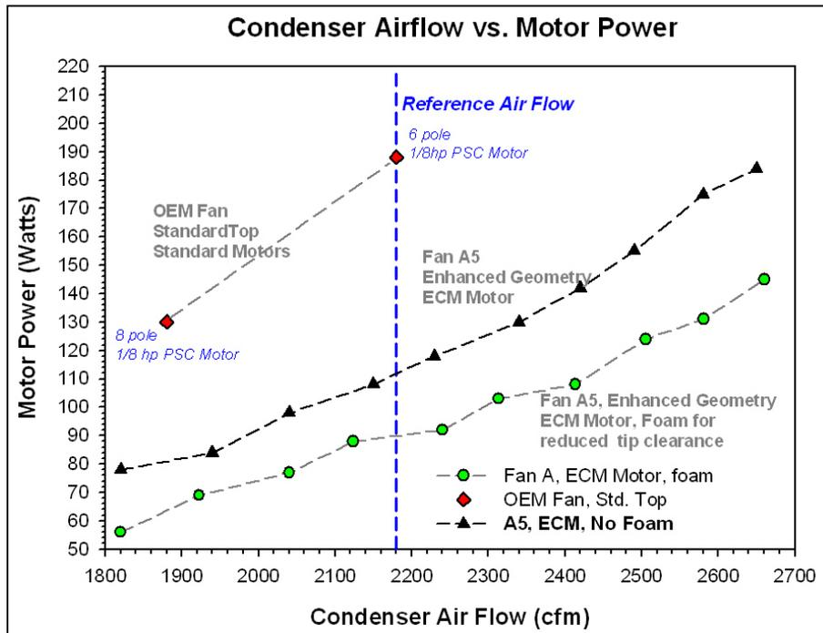
**Figure 9.** Impact on performance of Fan A5 used with elongated diffuser with and without tip clearance foam strip.
