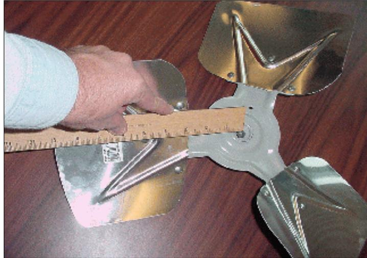
**Figure 2.** Stamped metal condenser fan blades for a 3-ton condenser
