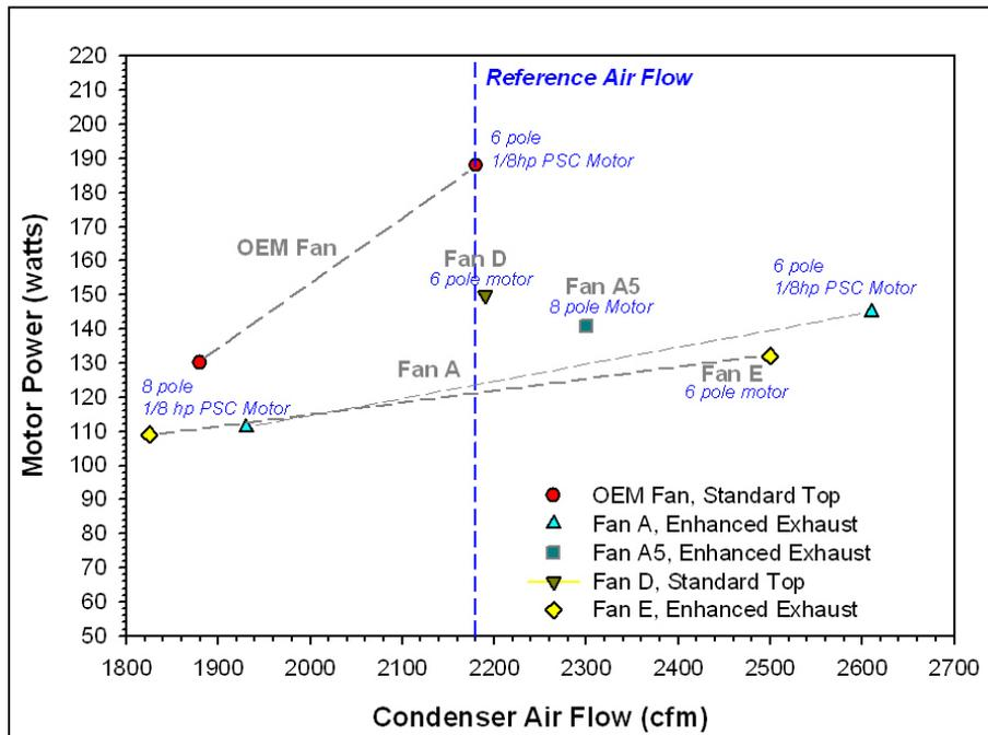
**Figure 7.** Performance of different fans with and without the enhanced diffuser against the original configuration
