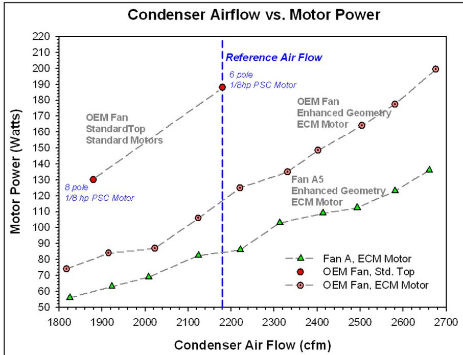
**Figure 8.** Impact of BDC motor and improved fan blades on condenser performance.
