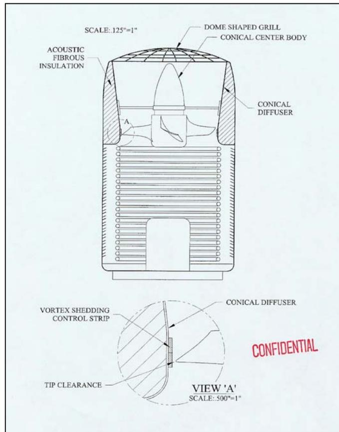
**Figure 6.** Diagram of the improved condenser fan with enhanced diffuser.
