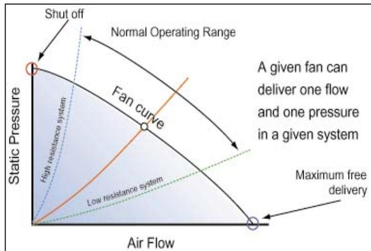
**Figure 3.** Illustration of fan law impacts on air flow in AC condenser
