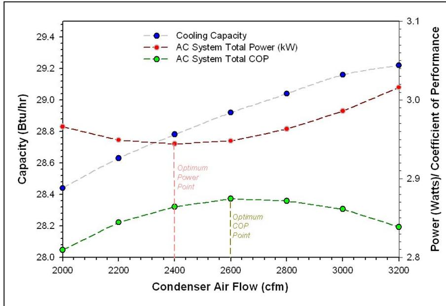
**Figure 4.** Evaluation of Optimum System Outdoor Air Flow for a Hypothetical 3-ton air conditioner
