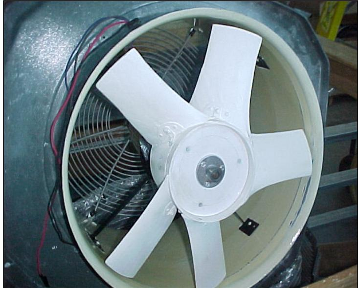
**Figure 5.** 19" Fan A5 with asymmetrical blade spacing.
