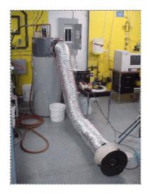
Figure 112 Airflow measurements using a Duct tester on heat pump cold air discharge side.
