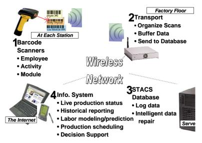
Figure 8 STACS system components and relationships.
