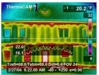
Figure 16 IR-scan showing metal trusses in precast walls. Temperature at the crosshairs is 20.2 °F. Overlaid temperature graph shows temperature variation of the surfaces at the white line running horizontally through the crosshairs.
