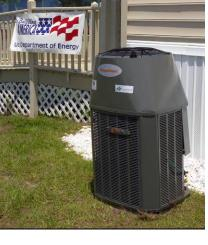
*Figure 98 Final test prototype with diffuser and fan.*
