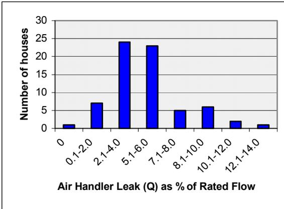
**Figure 5. Distribution of Q / Rated Flow for 9 Gas Furnace Cabinets and Cooling Coil Boxes**
