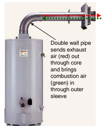
Direct Vent Gas Water Heater
