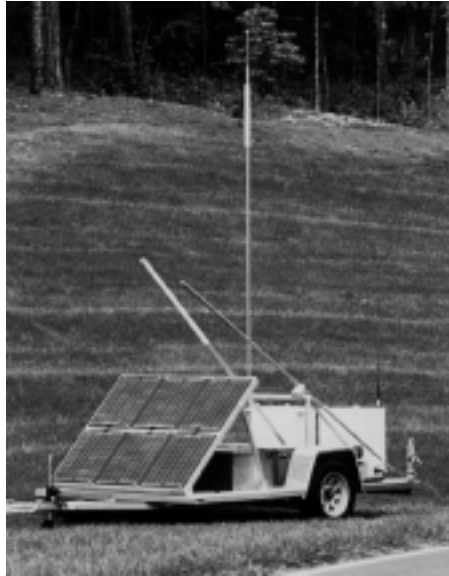
Figure 12.18 PV-Powered Radio Transmitter Along I-75
