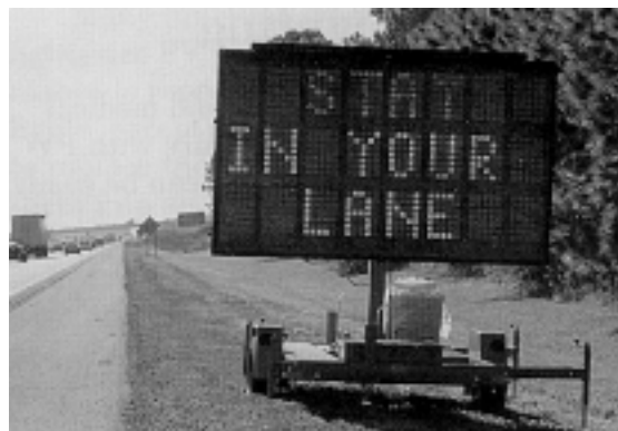
Figure 12.19 PV-Powered Changeable Message Sign
