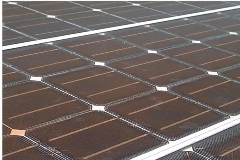
**Figure 30. ARCO Array Typical EVA Discoloration**
