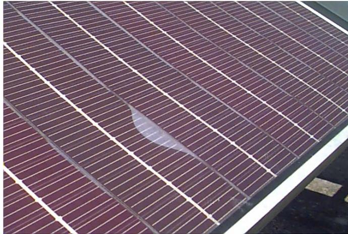
**Figure 27. Typical Sovonics Module Delamination**
