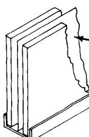
Heat mirror film is placed between two panes of glass.
