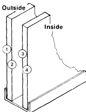
The low-e coating in insulated units faces the airspace and absorbs heat. Having the coating on surface 2 rather than surface 3 more effectively blocks the sun's heat from the house.
