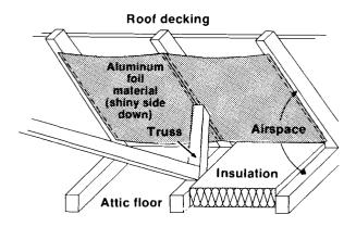
A radiant barrier can also be installed by stapling it to the bottom of the trusses.
