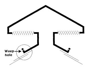
A ridge vent of this type is effective in resisting wind-driven water from backing up into openings. Weep hole is present in end flange.
