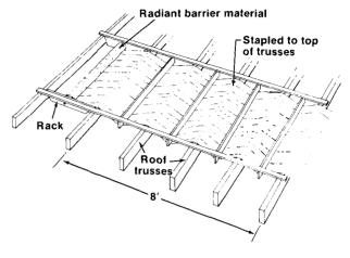
An easily-built radiant barrier installation rack.
