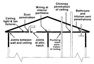
Major locations of air leakage between conditioned area and attic.
