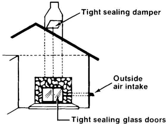
An energy-efficient fireplace has tight-sealing components.
