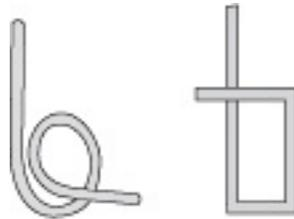
Embed the eyelet in the bottom of your car near the front (or use two eyelets--one near the front and one near the rear). The guide wire will pass through the eyelet to keep your car in its lane.
