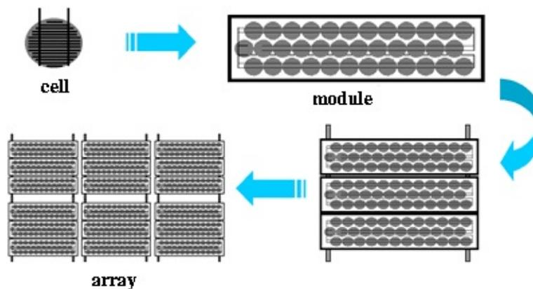
**Photovoltaic array** - The array which is made up of several photovoltaic modules converts sunlight directly into electric current. Like batteries, the current they produce is direct current (DC).
