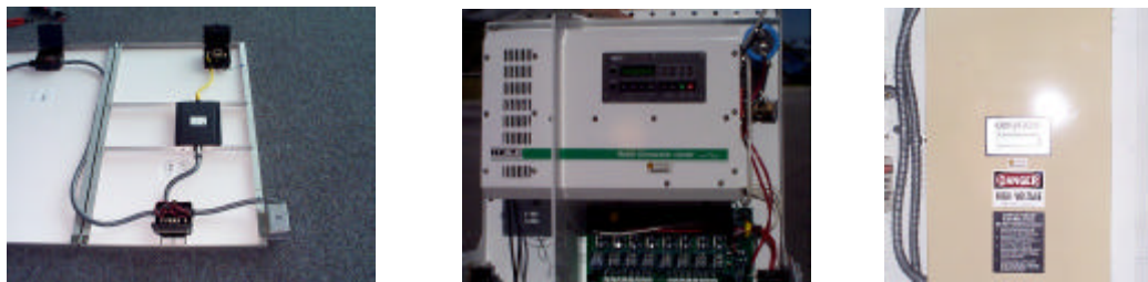
Figure 13. Several different inverters will be used in application experiments involving utility-interactive photovoltaic systems.
