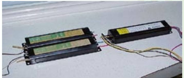
Figure 13. One electronic ballast replaces two magnetic ballasts.
